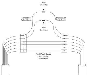
OTDR readings will be used to ensure proper installation and to troubleshoot faults. OTDR signature traces will be used for documentation and maintenance. An OTDR provides an indirect estimate of the loss of the cable plant, generally, more accurate or reliable values will be obtained by using an Optical Power Meter. For fibers that are identified in the Plans to be left unterminated, an OTDR shall be used to test end-to-end attenuation.
