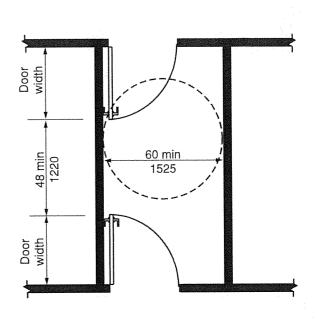
FIGURE 404.2.5(E) TWO DOORS OR GATES IN A SERIES - EXISTING BUILDINGS
