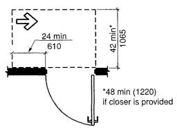
FIGURE 404.2.3.2(H) MANEUVERING CLEARANCE AT MANUAL SWINGING DOORS LATCH APPROACH - PUSH SIDE
