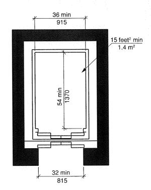
FIGURE 408.4.1(B) INSIDE DIMENSIONS OF LIMITED USE/LIMITED APPLICATION (LULA) ELEVATOR CARS EXISTING BUILDINGS - EXCEPTION 1
