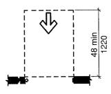
FIGURE 404.2.3.3(B) MANEUVERING CLEARANCES AT SLIDING AND FOLDING DOORS - FRONT APPROACH - EXISTING BUILDINGS FOOTNOTE 2
