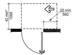
FIGURE 404.2.3.2(F) MANEUVERING CLEARANCE AT MANUAL SWINGING DOORS HINGE APPROACH - PUSH SIDE
