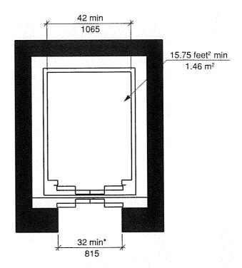
FIGURE 408.4.1(A) INSIDE DIMENSIONS OF LIMITED USE/LIMITED APPLICATION (LULA) ELEVATOR CARS - NEW BUILDINGS
