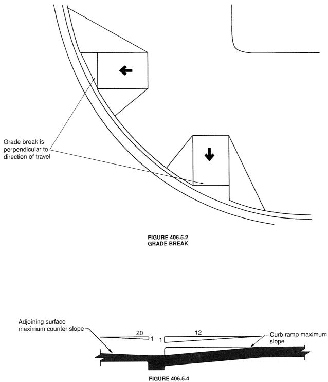
COUNTER SLOPE OF SURFACES ADJACENT TO CURB RAMPS
