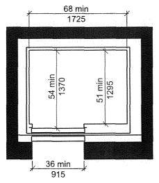
FIGURE 407.4.1(B) INSIDE DIMENSIONS OF ELEVATOR CARS SIDE (OFF-CENTERED DOOR) LOCATION
