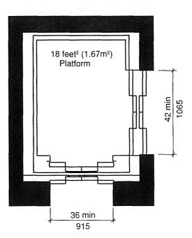
FIGURE 408.3.3(C) DOOR LOCATION FOR LIMITED USE/LIMITED APPLICATION (LULA) ELEVATORS - CAR WITH DOORS ON ADJACENT SIDES
