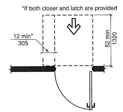
FIGURE 404.2.3.2(B) MANEUVERING CLEARANCE AT MANUAL SWINGING DOORS FRONT APPROACH - PUSH SIDE - NEW BUILDINGS
