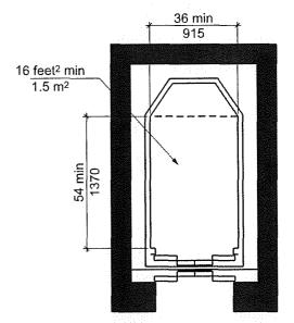
FIGURE 407.4.1(E) INSIDE DIMENSIONS OF ELEVATOR CARS EXISTING CAR CONFIGURATION
