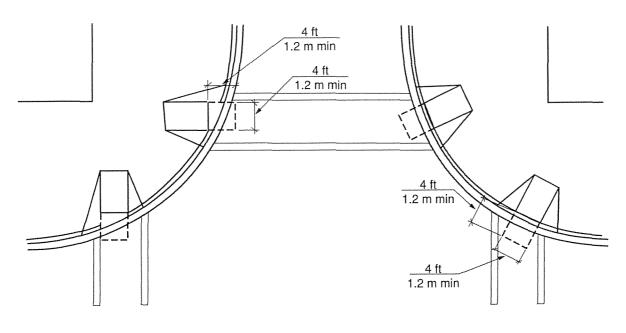
FIGURE 406.5.5 CLEAR SPACE AT BOTTOM OF CURB RAMPS AND BLENDED TRANSITIONS
