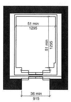
FIGURE 408.4.1(C) INSIDE DIMENSIONS OF LIMITED USE/LIMITED APPLICATION (LULA) ELEVATOR CARS EXISTING BUILDINGS - EXCEPTION 2
