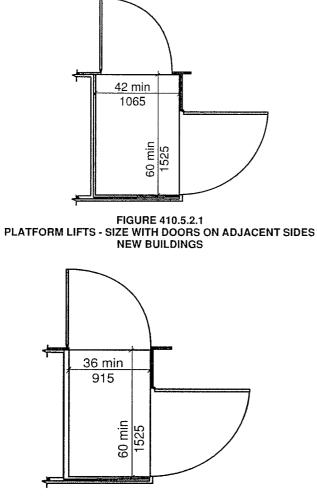
FIGURE 410.5.2.2 PLATFORM LIFTS - SIZE WITH DOORS ON ADJACENT SIDES EXISTING BUILDINGS
