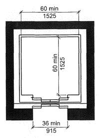
FIGURE 407.4.1(D) INSIDE DIMENSIONS OF ELEVATOR CARS ANY DOOR LOCATION
