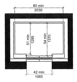
FIGURE 407.4.1(A) INSIDE DIMENSIONS OF ELEVATOR CARS - CENTERED DOOR LOCATION
