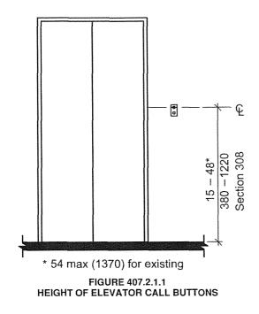
**407.2.1.4 Location.** The call button that designates the up direction shall be located above the call button that designates the down direction.
