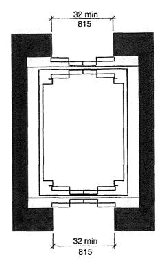
FIGURE 408.3.3(B) DOOR LOCATION FOR LIMITED USE/LIMITED APPLICATION (LULA) ELEVATORS - CAR WITH DOORS ON OPPOSITE SIDES
