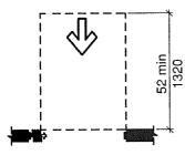
FIGURE 404.2.3.3(A) MANEUVERING CLEARANCES AT SLIDING AND FOLDING DOORS - FRONT APPROACH - NEW BUILDINGS
