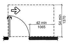
FIGURE 404.2.3.2(E) MANEUVERING CLEARANCE AT MANUAL SWINGING DOORS HINGE APPROACH - PULL SIDE
