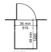
FIGURE 410.5.1.2 PLATFORM LIFTS - SIZE WITH SINGLE DOOR OR DOORS ON OPPOSITE ENDS - EXISTING BUILDINGS
