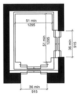
FIGURE 408.3.3(D) DOOR LOCATION FOR LIMITED USE/LIMITED APPLICATION (LULA) ELEVATORS - CAR WITH DOORS ON ADJACENT SIDES - EXCEPTION
