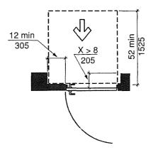
FIGURE 404.2.3.5(C) RECESSED DOORS AND GATES - NEW BUILDINGS PUSH SIDE - DOOR PROVIDED WITH BOTH CLOSER AND LATCH
