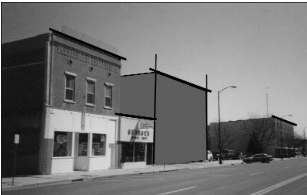
The roof form of new commercial buildings should match that of other historic commercial buildings in the area
