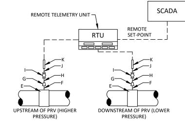
PRESSURE TRANSDUCER INSTALLATION
