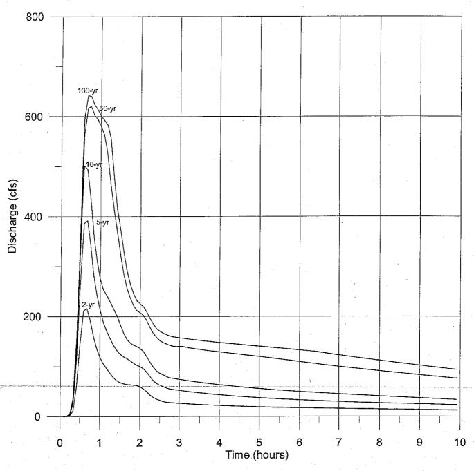
Figure D.6 Flood Hydrographs at C Street (35th Avenue Outfall Channel) Future Condition (EPA SWMM Node 426)
