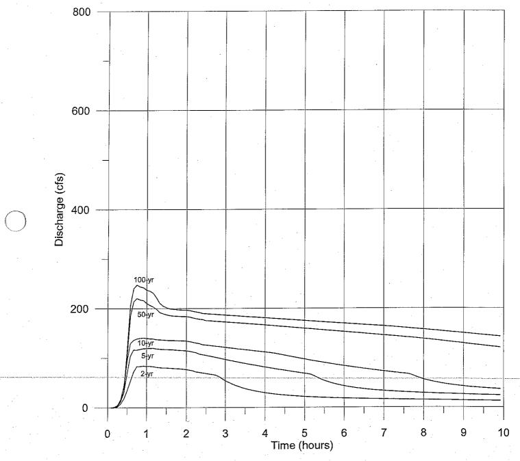
Figure D.9 Flood Hydrographs at C Street (35th Avenue Outfall Channel) Proposed Condition (EPA SWMM Node 426)
