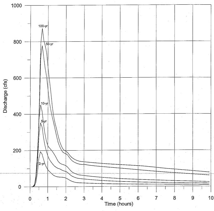
Figure D.2 Flood Hydrographs at 35th Avenue and 4th Street (all flows) Existing Condition (EPA SWMM Node 420)
