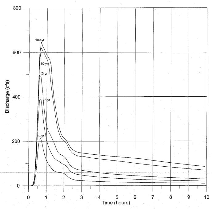
Figure D.3 Flood Hydrographs at C Street (35th Avenue Outfall Channel) Existing Condition (EPA SWMM Node 426)
