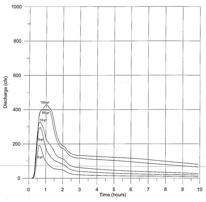
Figure D.8 Flood Hydrographs at 35th Avenue and 4th Street (all flows) Proposed Condition (EPA SWMM Node 420)
