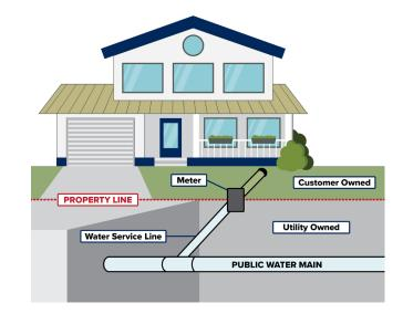
As shown in this diagram, the city owns the service line that runs from the main water line to the property line. The customer owns the service line, which may include the curb stop and water meter, that runs from the property line into their house.
