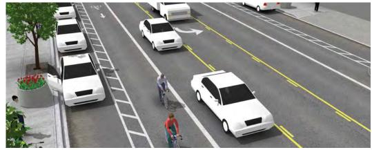
Figure 4-3: Typical buffered bike lanes with parking-side buffer
