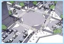
Figure 4-7: Protected intersection concept
