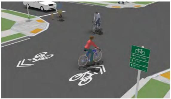
Figure 2-8: Typical bike boulevard marking and signage
