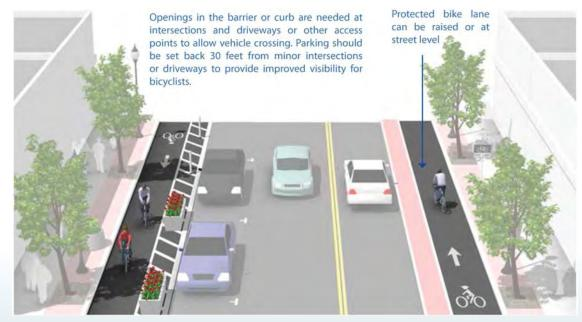
Figure 2-14: Typical protected bike lane cross section with and without parking
