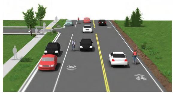
Figure 2-6: Typical shared lane cross section with and without parking
