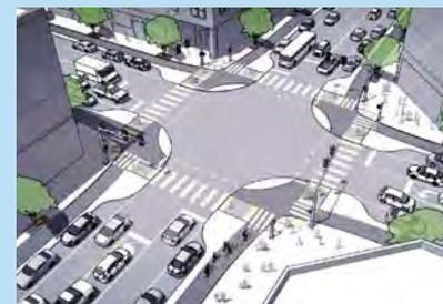
Figure 4-7: Protected intersection concept
