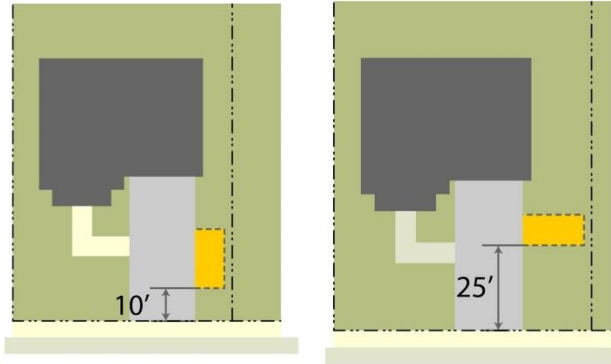
Figure 24-5-12 Accessory Parking Pad To meet parking requirements, accessory parking pads may be approved by alternative compliance provided they minimize impacts on the streetscape and adjacent property. (24-503.b.5.(c))
