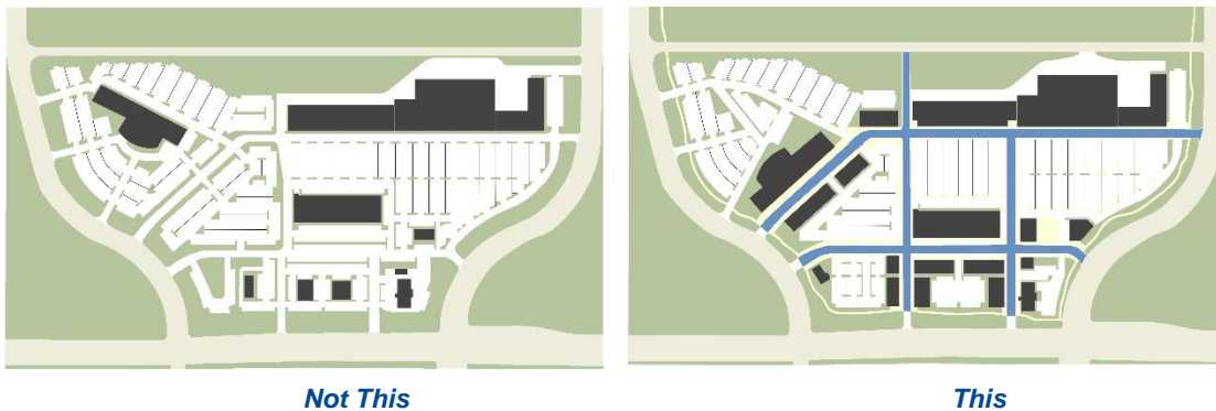
Figure 24-7-1: Internal access streets.
