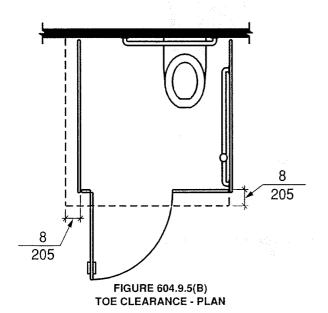
604.9.5.1 Toe clearance at wheelchair accessible toilet compartments. The front partition and at least one side partition of wheelchair accessible toilet compartments shall provide a toe clearance of 12 inches (305 mm) minimum above the floor and extending 8 inches (205 mm) beyond the compartment side face of the partition, exclusive of partition support members.
