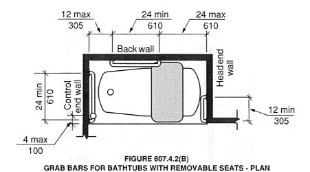
**607.5** Controls. Controls, other than drain stoppers, shall be provided on an end wall, located between the bathtub rim and grab bar, and between the open side of the bathtub and the centerline of the width of the bathtub. Controls shall comply with Section 309.4.
