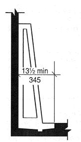
FIGURE 605.2(B) **HEIGHT AND DEPTH OF URINAL** STALL TYPE
