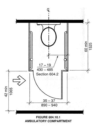
**604.10.2 Size.** The minimum area of an ambulatory accessible toilet compartment shall be 60 inches (1525 mm) minimum in depth and a width of 35 inches (890 mm) minimum and 37 inches (940 mm) maximum.
