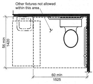
**FIGURE 604.3** SIZE OF CLEARANCE FOR WATER CLOSET
